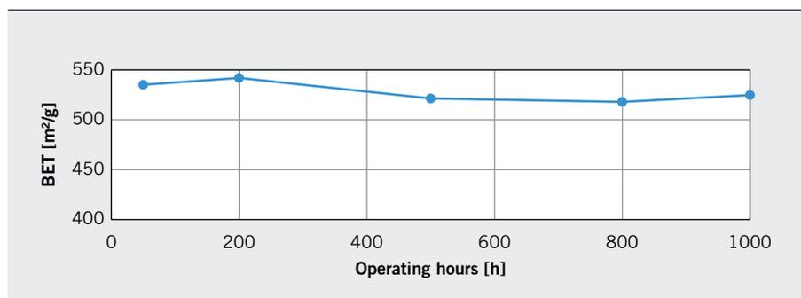
**FIGURE 6** BET of the SCR throughout the operating time of 1000 h
