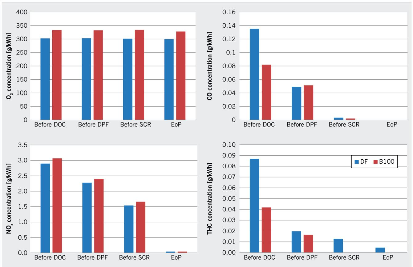
FIGURE 4 Exhaust gas concentrations for DF and B100 at load point 6 (n = 1600 rpm, M = 370 Nm) (© University of Rostock)
