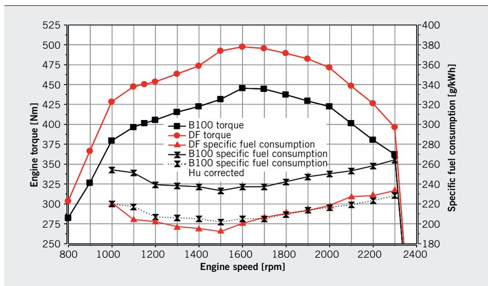
FIGURE 3 Torque curve and fuel consumption of DF and B100 (© University of Rostock)
