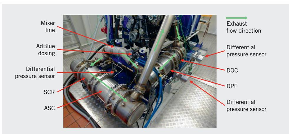
**FIGURE 1** Setup of the exhaust aftertreatment system of the engine on the test bench (© University of Rostock)
