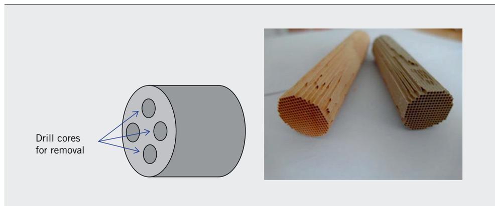
FIGURE 2 Representation of drill core removal and cores from the DOC and SCR (© University of Rostock)
