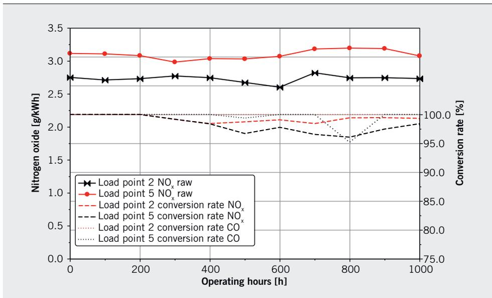
FIGURE 5 Nitrogen oxide concentrations and conversion rates throughout the operation time of 1000 h for B100 operation (© University of Rostock)
