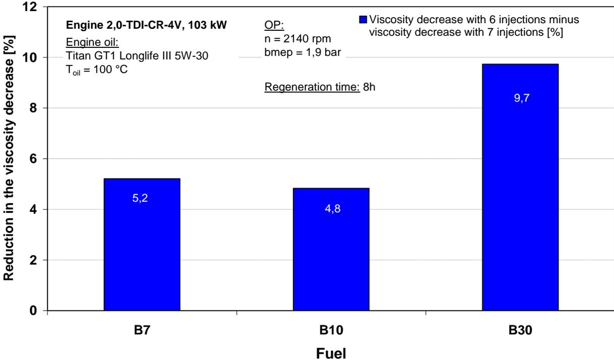
Figure 6-9: Reduction in the viscosity decrease through the split late post-injection (variant V5), in comparison to the series application “new” with 6 injections per cycle
