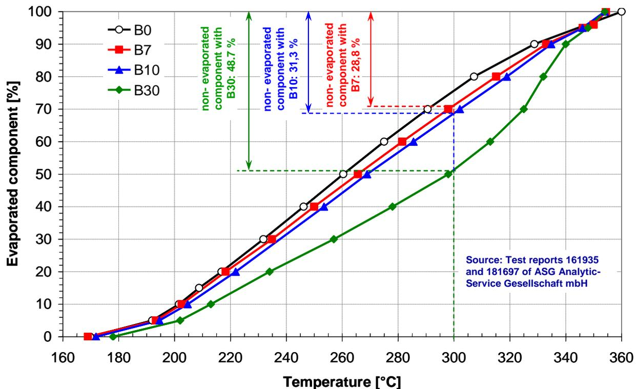
**Figure 3-1:** Boiling curves of the fuels B0, B7, B10 and B30
