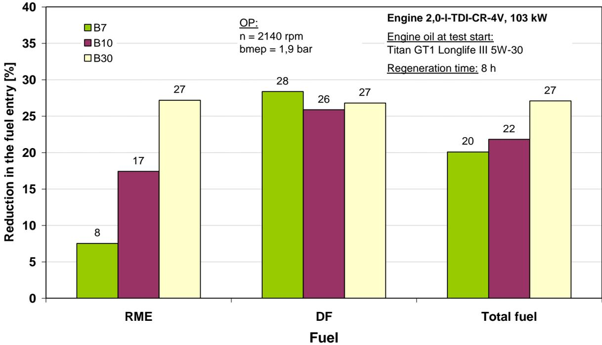
Figure 6-8: Reduction in the fuel entry through the split late post-injection (variant V5), in relation to the series application "new" with 6 injections per cycle
