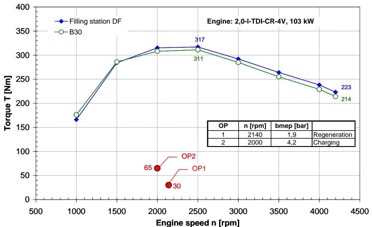
**Figure 4-5:** Operating points and full load curve of the engine with B10
