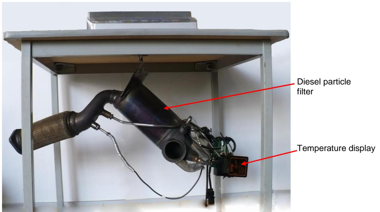
Figure 4-5: Weighing the diesel particle filter
