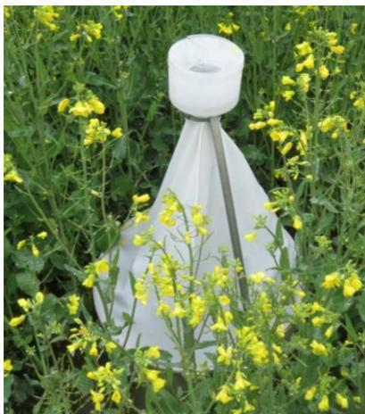
**Figure 4:** Emergence trap; base rings of  $0.25 \text{ m}^{-2}$  with fabric tents and openings on top closed with a plastic container. In the present experiment plastic bags were used instead of containers to trap emerging insect pests.
