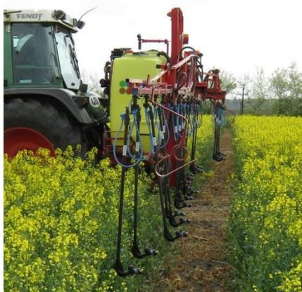
**Figure 2:** Droplegs with spray nozzles hanging approx. 40 cm below the crop canopy of a flowering OSR field (HAUSMANN 2017).
