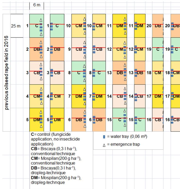
**Figure 1:** Experimental design for the field trial conducted in a randomized block design; plot descriptions; red lines mark cross lines within the plots; water trays and emergence traps are visualized.
