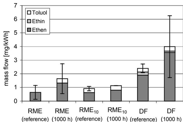
Figure 13. Specific emission for alkenes, alkynes and aromatics.
