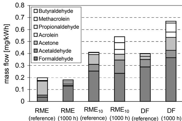
Figure 14. Specific emission for aldehydes and ketones.
