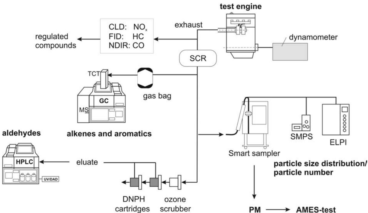
Figure 2. Scheme of the emission test stand.
