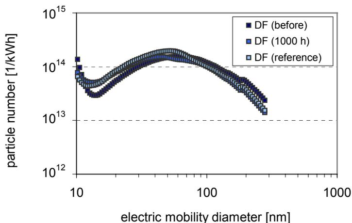
Figure 12. Size distribution of particles of DF (SMPS).
