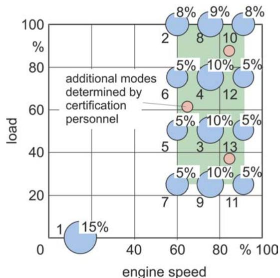
Figure 1. Modes of the ESC test.
