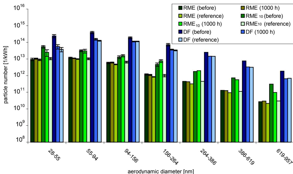
Figure 8. Size distribution of particles (ELPI).
