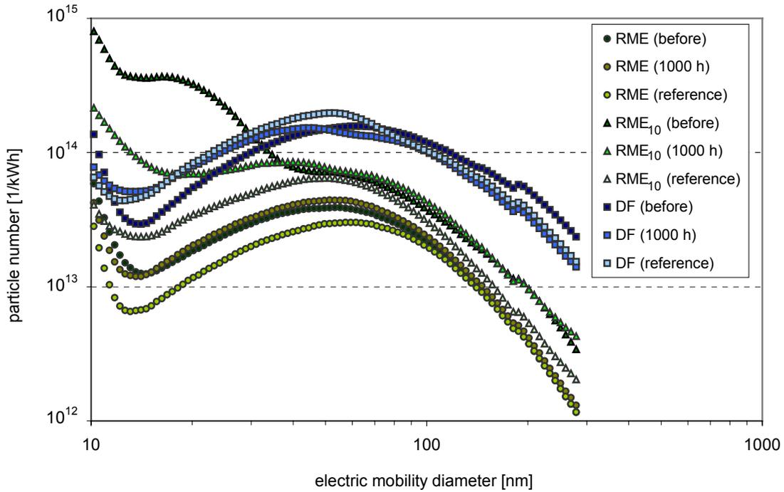
Figure 9. Size distribution of particles with respect to number of particles (SMPS).
