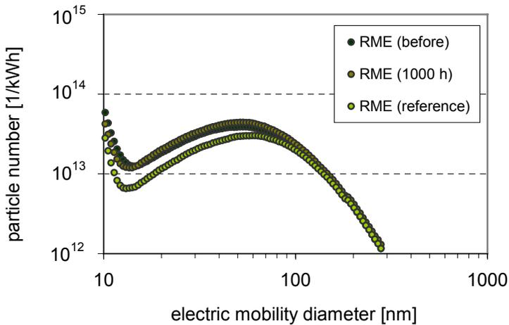
Figure 10. Size distribution of particles of RME (SMPS).
