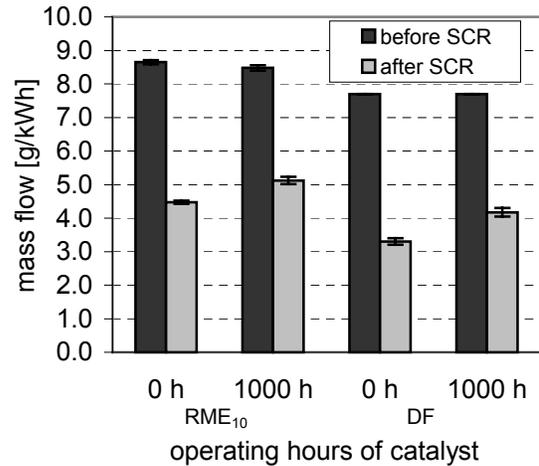
Figure 4. Specific NO<sub>x</sub> emission.
