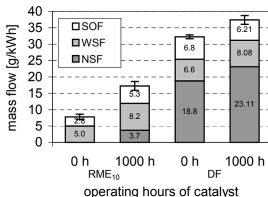
Figure 7. Composition of particulate matter.
