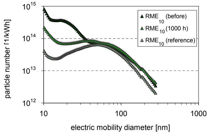
Figure 11. Size distribution of particles of  $RME_{10}$  (SMPS).
