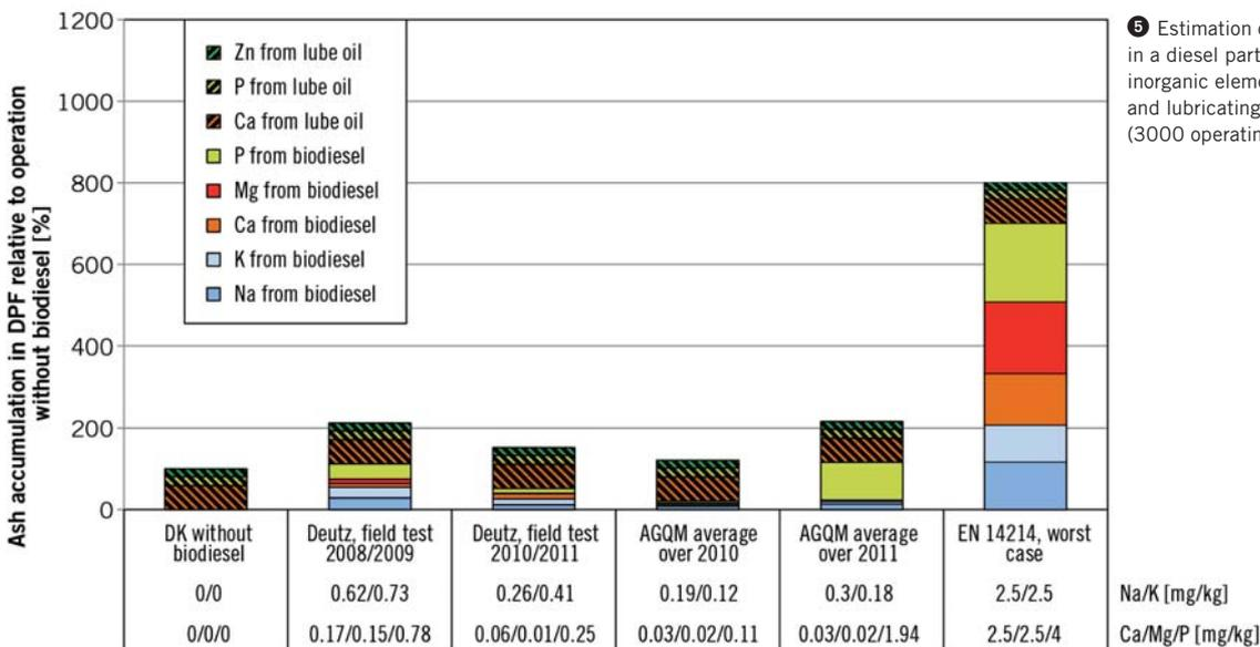
⑤ Estimation of ash contaminant in a diesel particle filter caused by inorganic elements from biodiesel and lubricating oil at tractor operation (3000 operating hours)
