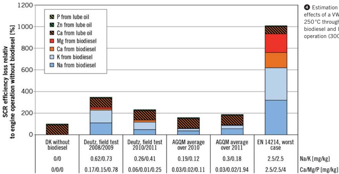
④ Estimation of the contaminant effects of a VWT-SCR coated catalyst at 250°C through inorganic elements from biodiesel and lubricating oil at tractor operation (3000 operating hours)
