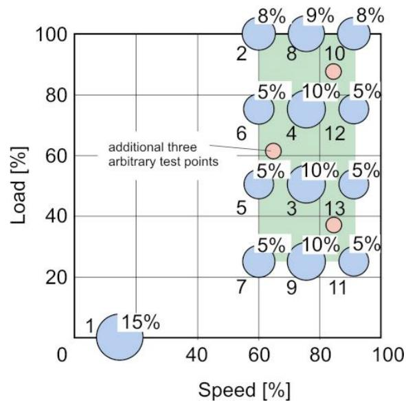
Abb. 2-1: ESC test cycle
