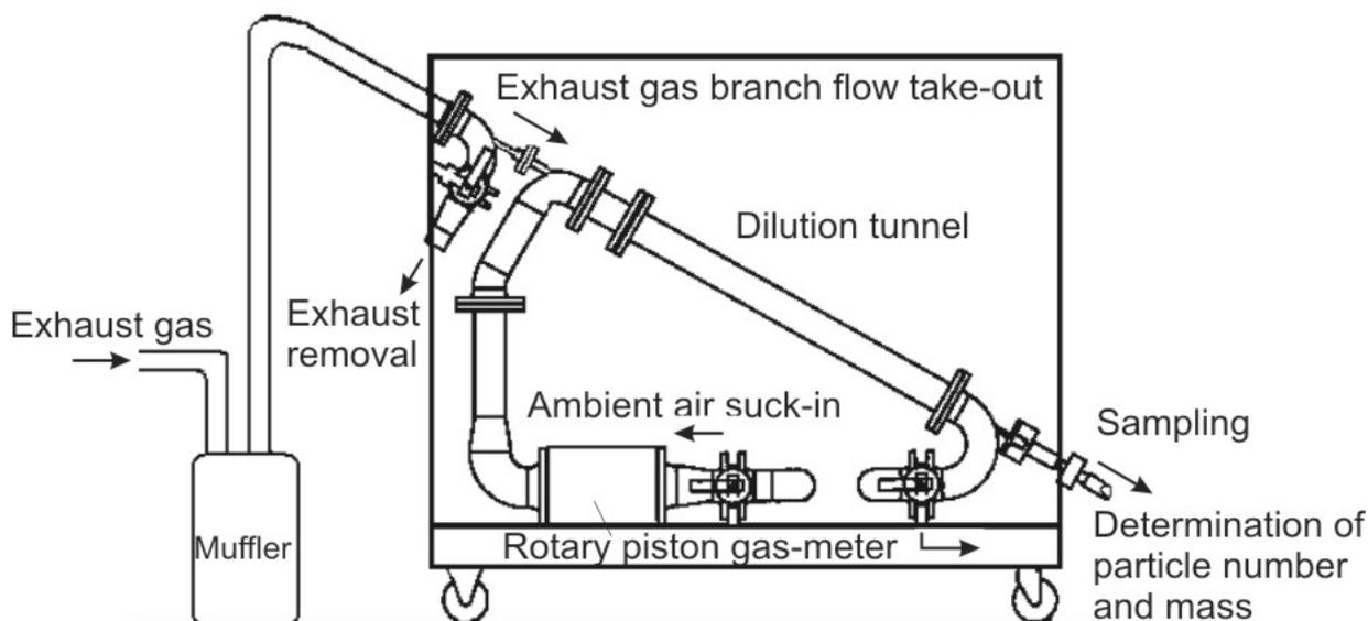
Fig. 2-3: Schematic presentation of the exhaust gas dilution tunnel
