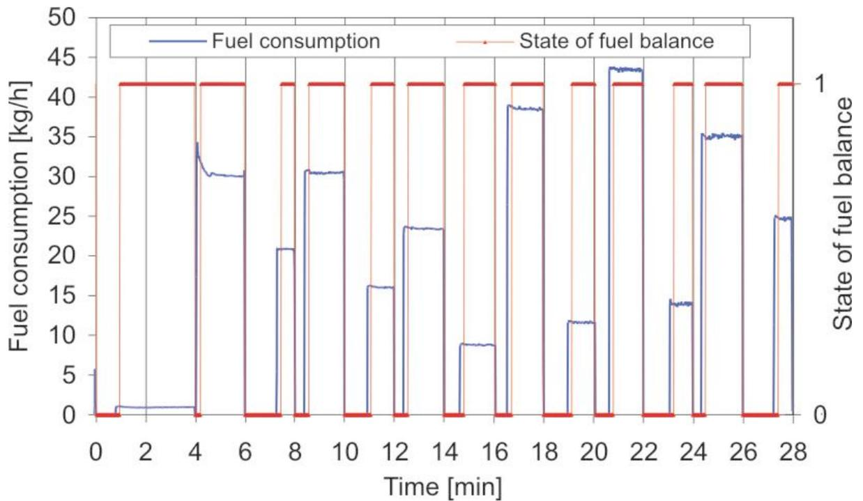
Fig. A-8: Exemplary course of the fuel consumption; measurements only take place during scale status “1,” at status “0” the scale is refilled. (Run SMDS23, GTL)
