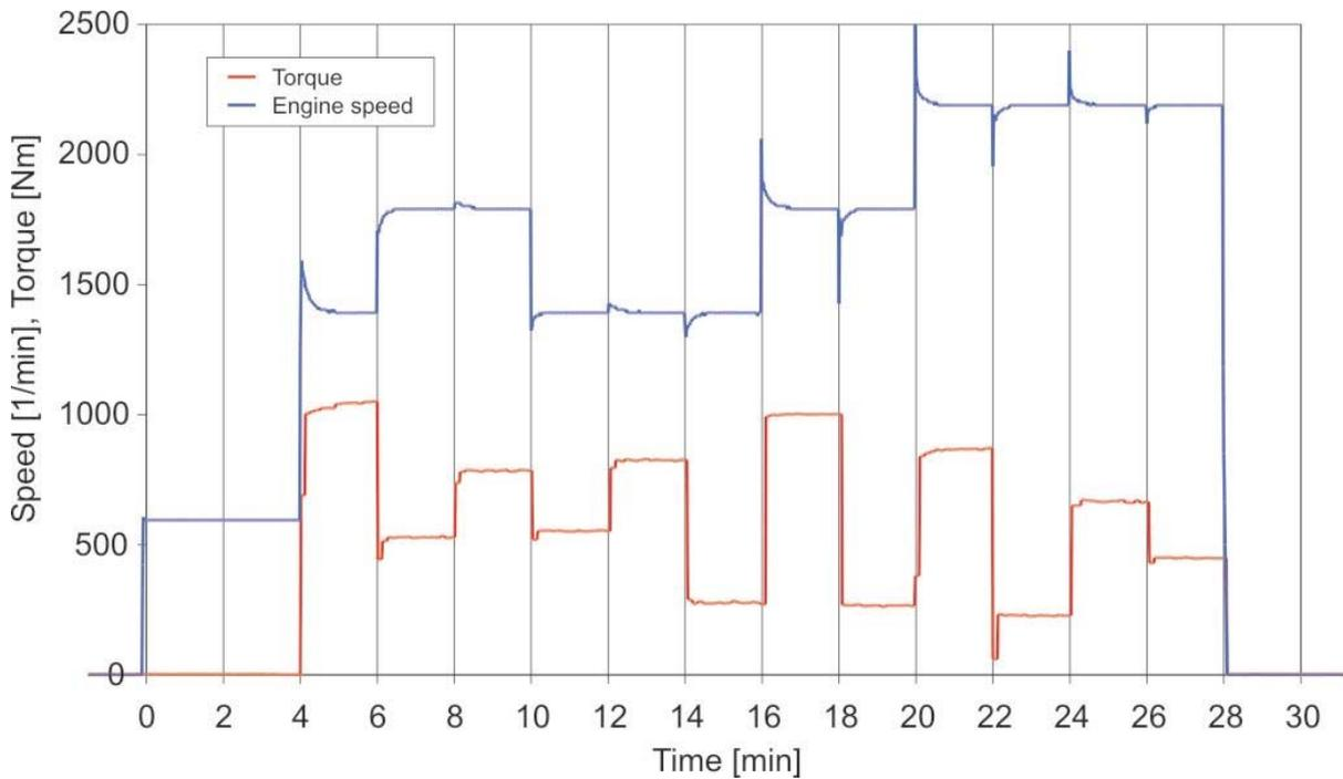
Abb. 2-2: Actual course of speed and torque (Run SMDS06, PDF)
