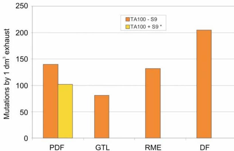
Fig. 3-18: Mutagenicity of particulate matter extracts in strain TA100 (\* the number of mutations increased significantly only for PDF)
