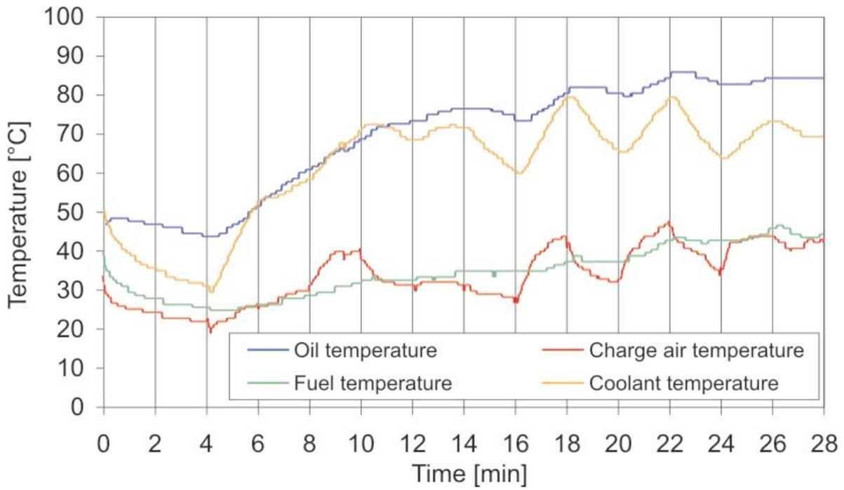
Fig. A-5: Exemplary course of the charge air, coolant, oil and fuel temperatures (Run SMDS23, GTL)
