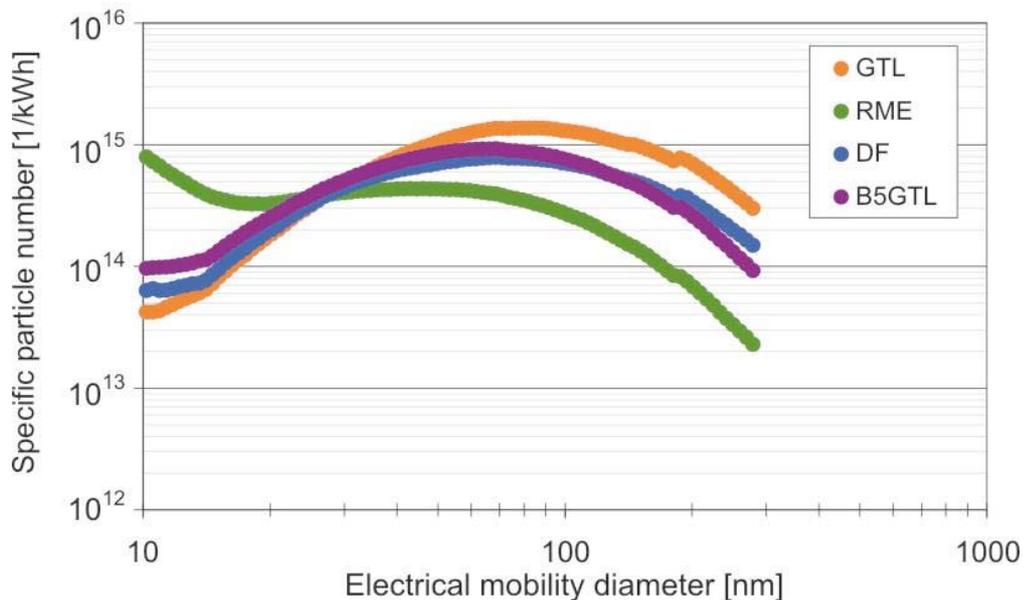
Fig. 3-9 Specific particle count distribution in crude exhaust gas (SMPS – 2<sup>nd</sup> test series)
