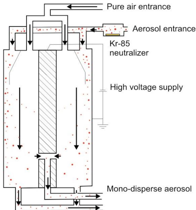
Fig. 2-4: Simplified presentation of a DMA
