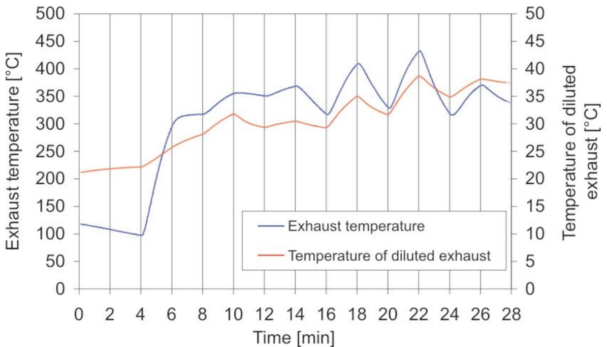
Fig. A-4: Exemplary course of the exhaust gas temperature and the temperature of the diluted exhaust gas in the dilution tunnel (Run Ref118, GTL)
