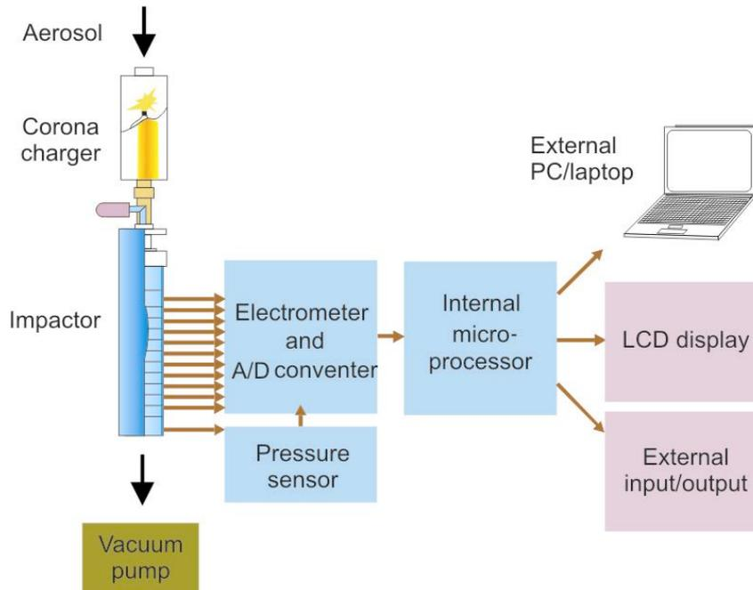
Fig. 2-6: Functioning principle of ELPI (Dekati, 2002)
