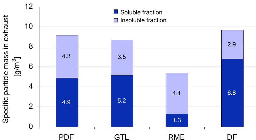
Fig. 3-16: Soluble and insoluble particulate matter fractions in raw exhaust gas
