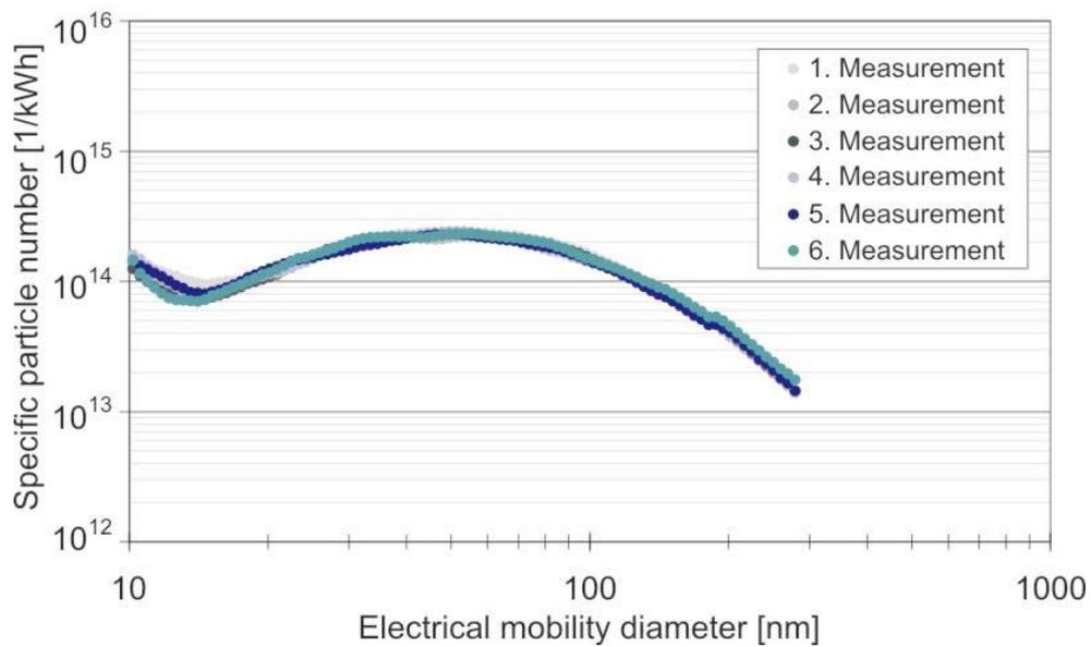
Fig. 3-11: Single measurements for GTL (SMPS – 1<sup>st</sup> test series)
