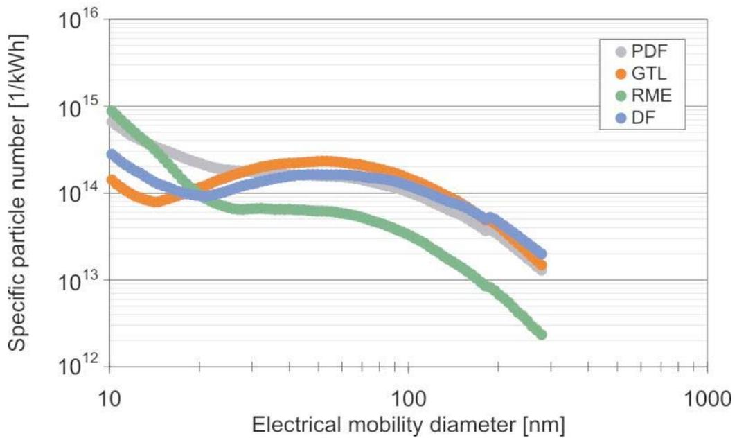
Fig. 3-8: Specific particle number distribution in crude exhaust gas (SMPS – 1<sup>st</sup> test series)
