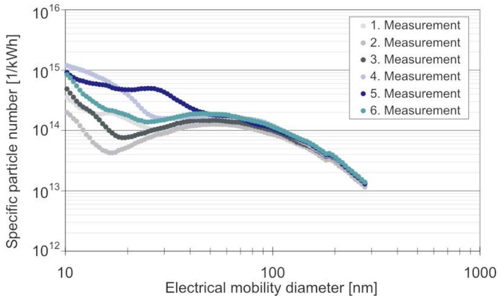
Fig. 3-10: Single measurements for PDF (SMPS – 1<sup>st</sup> test series)
