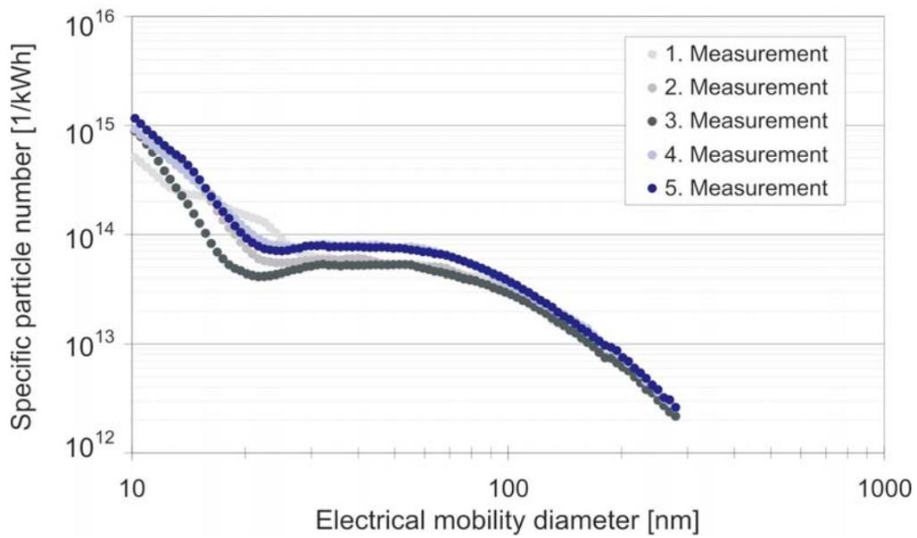
Fig. 3-12: Single measurements for RME (SMPS – 1<sup>st</sup> test series)
