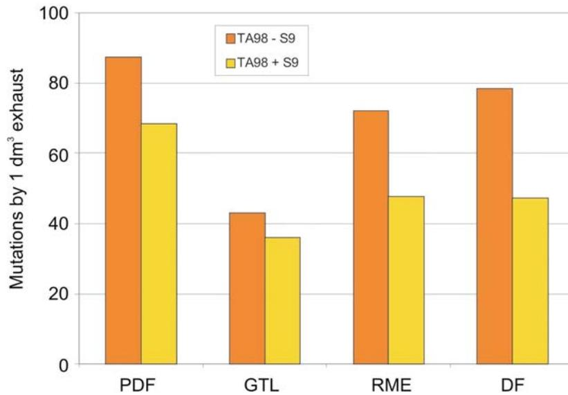
Fig. 3-17: Mutagenicity of particulate matter extracts in strain TA98
