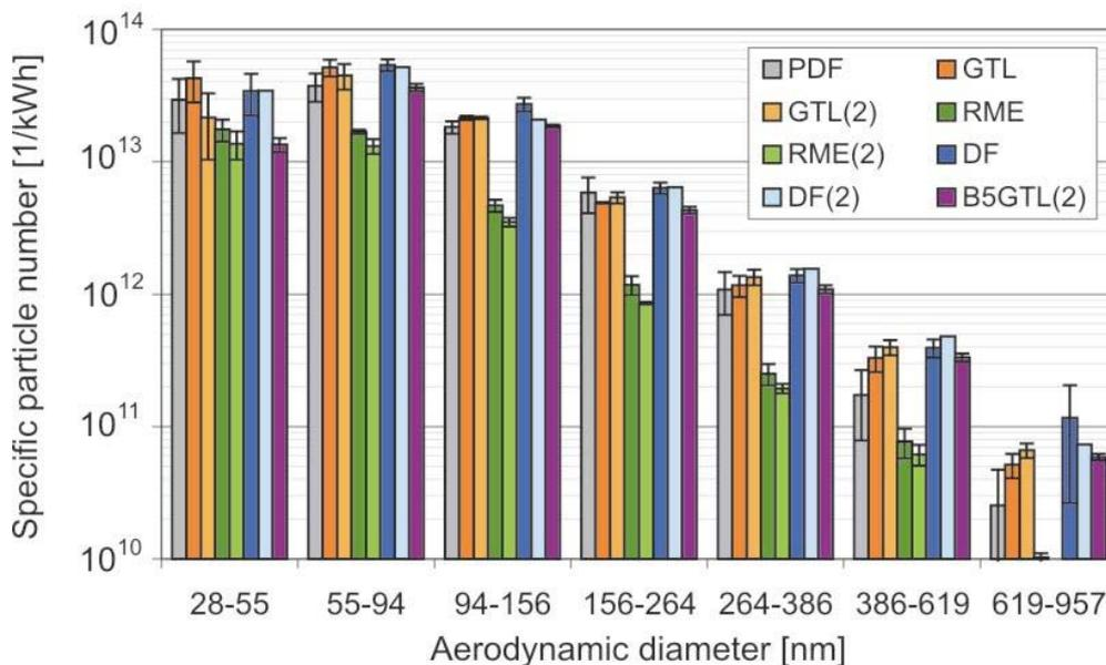
Fig. 3-15: Specific particle number distribution in raw exhaust gas (ELPI)
