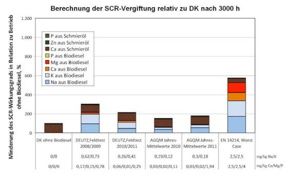
Illustration 14: Estimate of the poisoning effects of a VWT-SCR-coating catalytic converter at 250°C by inorganic elements from Biodiesel and lubricating oil during tractor operation (3000 h).
