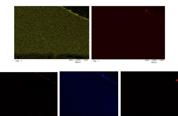
Illustration 7: REM-images with EDX-Mapping of the elements sulphur (top left), calcium (top right), sodium (bottom left), phosphorus (bottom centre), potassium (bottom right) (Source: Umicore)
