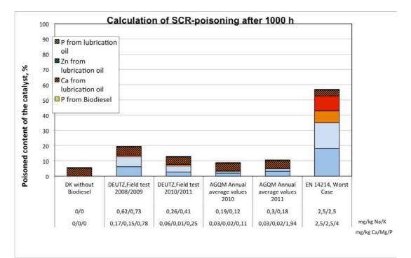
Illustration 13: Estimate of the poisoning effects of a VWT-SCR-coating catalytic converter at 250°C by inorganic elements from Biodiesel and lubricating oil during tractor operation (1000 h).
