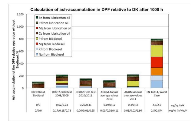
Illustration 15: Estimate of the ash burden in a Diesel particle filter by inorganic elements from Biodiesel and lubrication oil in tractor operation (1000 h).
