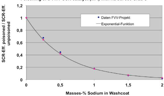
Poisoning of a VWT-SCR-catalyst (MFI) with Na bei 350 Grad C
