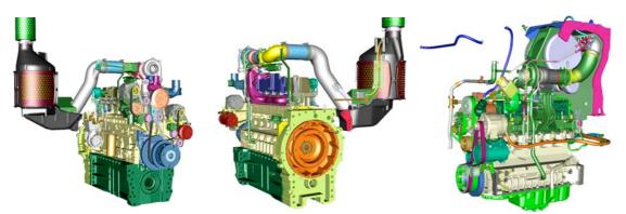
Illustration 3: Design TCD 7.8 L6 (Fendt X 911) with cone-SCR-catalytic converter (left/centre) and TCD 6.1 L6 (Fendt X 850/X 711) with hood-SCR-catalytic converter (right)
