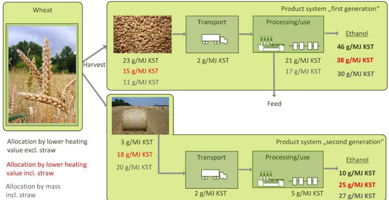
Figure 5 Overview of the GHG emissions from the production and utilisation of ethanol based on wheat grain and wheat straw with consideration to various allocation approaches for straw as a co-product (when using natural gas in a conventional boiler; allocation in accordance with lower calorific value and mass, all calculations based on the typical values in Annex V of EU RED)
