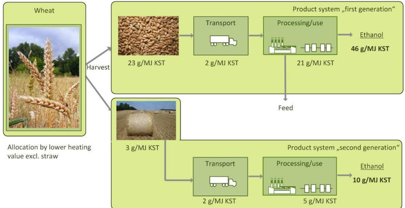
Figure 3 disaggregated typical GHG emissions for the production of ethanol based on wheat grain (when using natural gas in a conventional boiler) and wheat straw (in accordance with Annex V EU RED)
