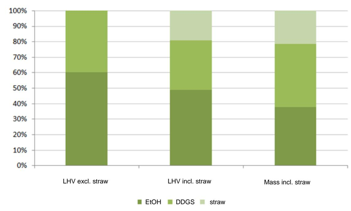
Figure 6 Relative proportion of the total emissions from the 'ethanol from wheat grain' pathway for the various products with different allocation approaches (LHV = lower calorific value)
