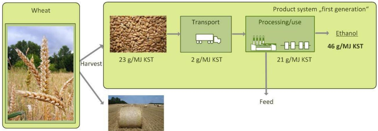
Figure2 disaggregated typical GHG emissions for the production of ethanol based on wheat grain (when using natural gas in a conventional boiler; in accordance with Annex V EU RED)
