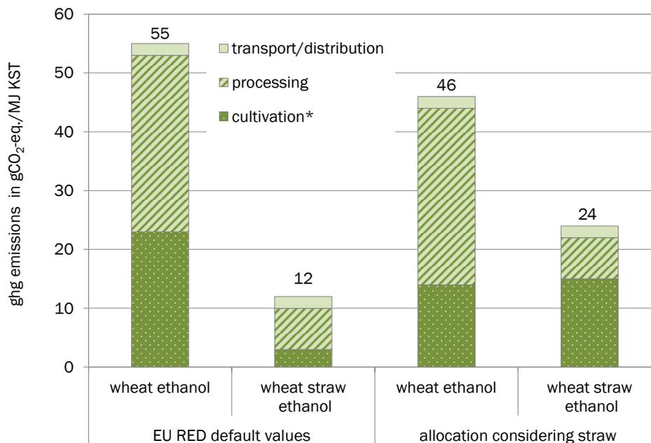
Figure 7 Comparison of the typical values for ethanol from wheat grain and wheat straw (when using natural gas in a conventional boiler; from Annex V of EU RED) and the GHG emissions of both pathways based on the new calculations performed considering straw as a co-product
