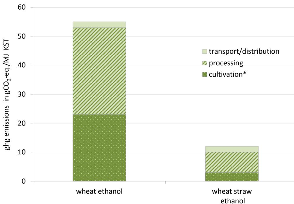
Figure 1 typical GHG emissions for ethanol based on wheat and wheat straw (in accordance with Annex V EU RED); \* = in the case of straw, the balance begins with straw gathering; agricultural production processes are not included
