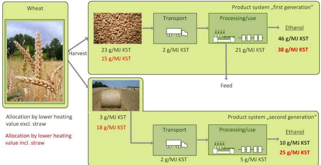
Figure 4: GHG emissions from the production and utilisation of ethanol based on wheat and wheat straw with consideration of straw as a co-product (when using natural gas in a conventional boiler, allocation in accordance with lower calorific value, all calculations based on the typical values in appendix V of EU RED)
