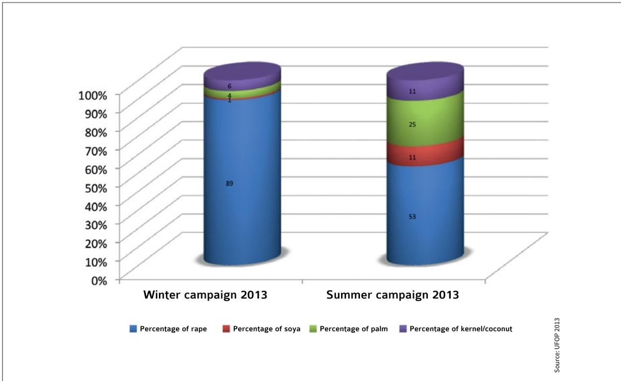
Figure 3: Raw material mix in the analysed biodiesel components
