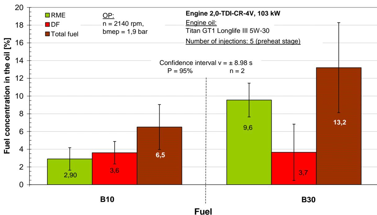
**Figure 6-10:** Fuel concentration in the engine oil after 8 hours engine operation in preheat mode with 5 injections per cycle at OP1 with B10 and B30
