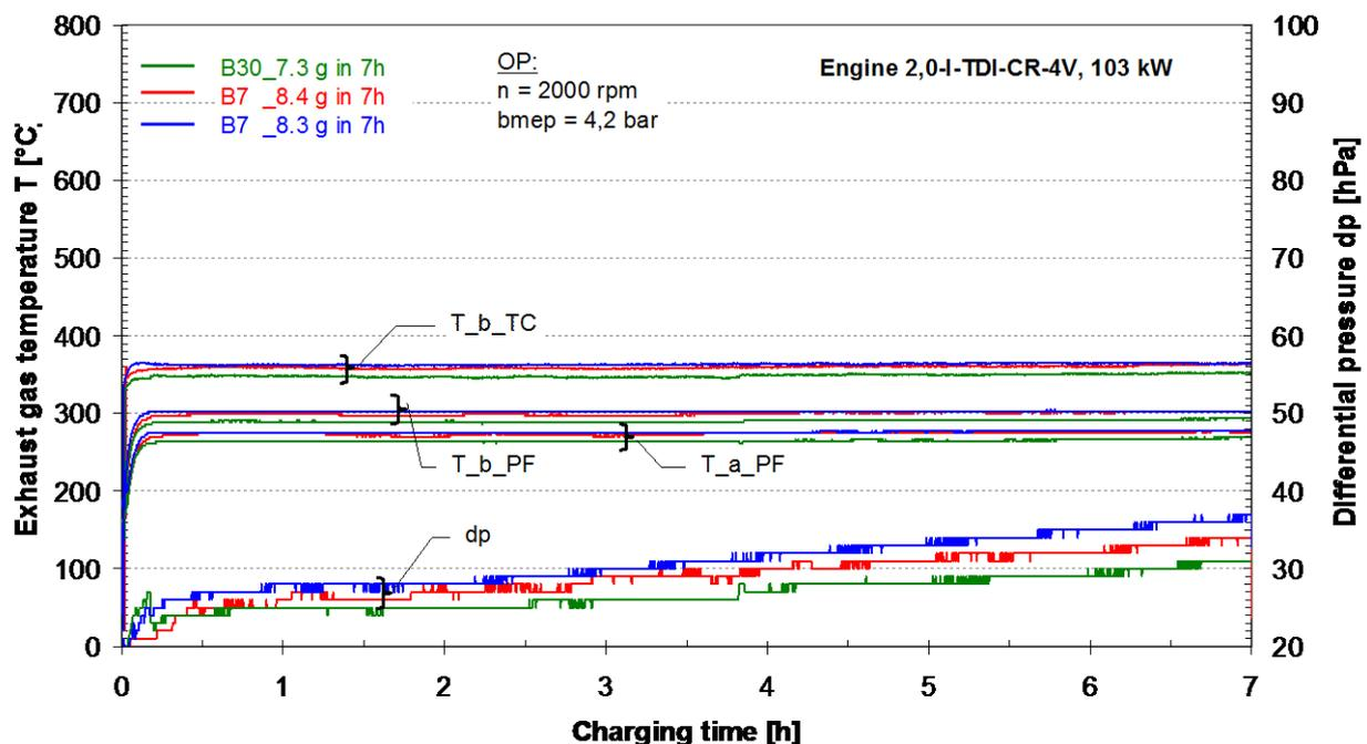
**Figure 6-14:** Exhaust gas temperatures and differential pressure of the DPF when charging the filter during engine operation at OP2 with B7 and B30
