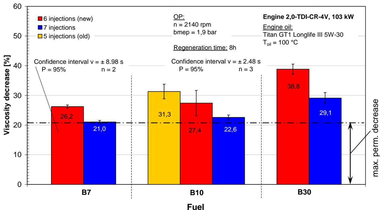
**Figure 6-7:** Decrease in the oil viscosity at 100 °C in regeneration mode over 8 hours at engine operation with 5, 6 and 7 injections (variant V5) with the fuels B7, B10 and B30
