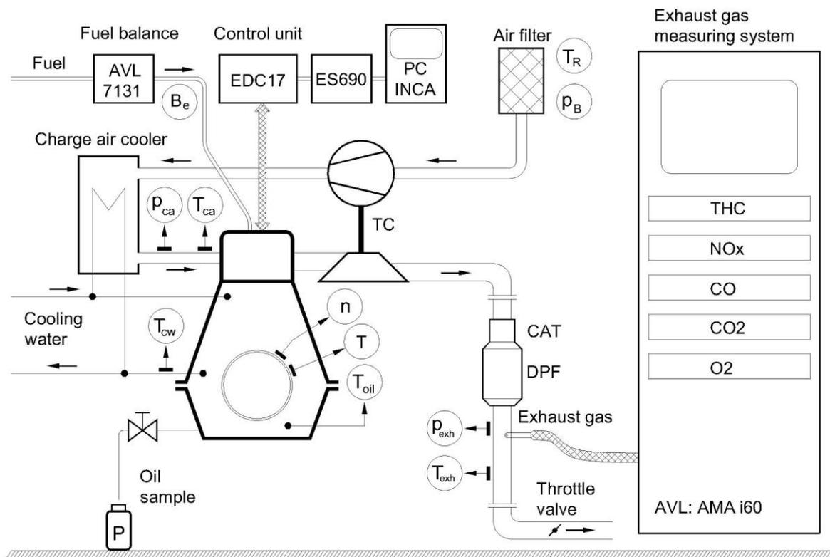
**Figure 4-2:** Engine test bench with exhaust gas after-treatment and measuring system
