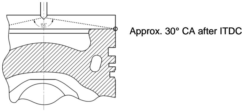
**Figure 6-1:** Crank angle limit for avoiding the jet impingement on the cylinder wall
