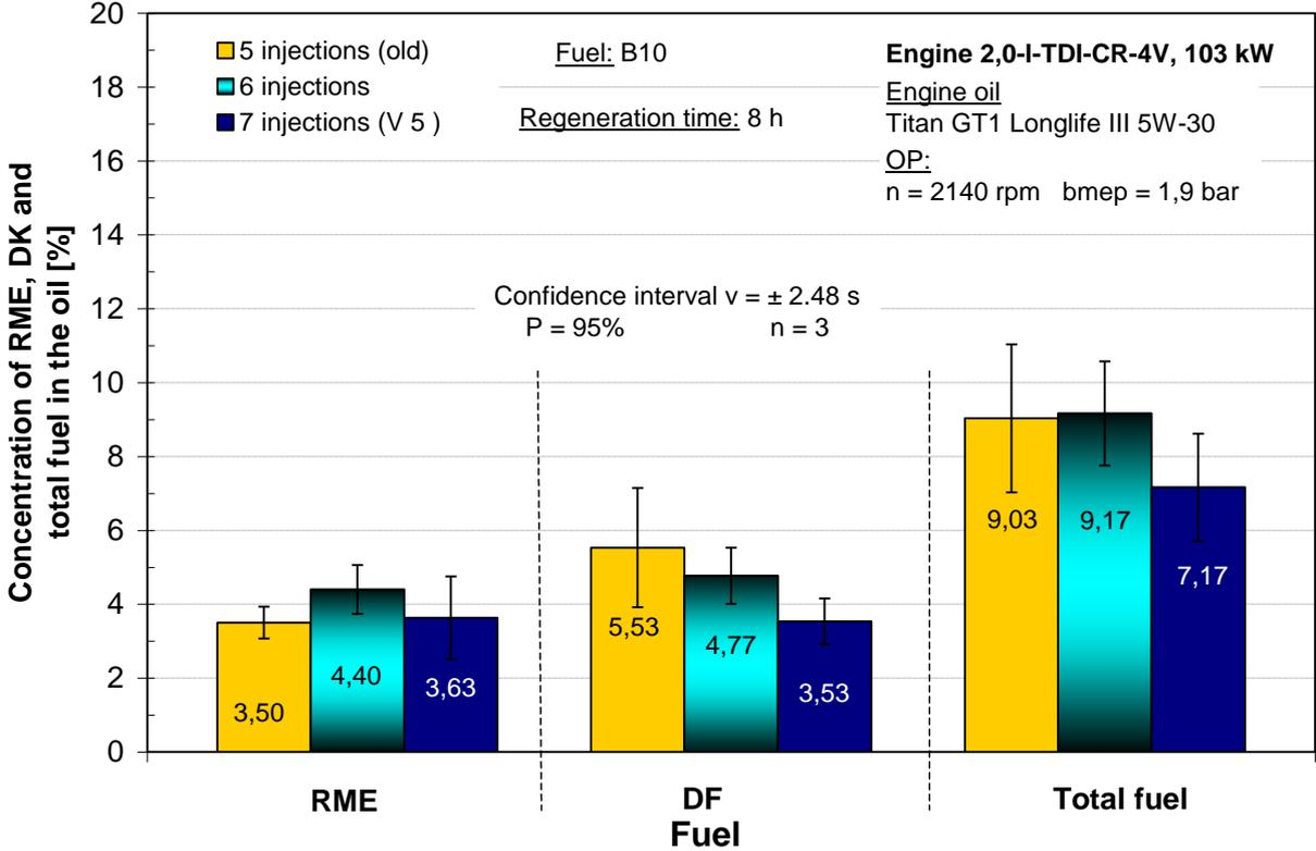
Figure 6-6: Concentration of total RME, DF and total fuel in the engine oil after 8 hours engine operation in regeneration mode with 5, 6 and 7 injections per cycle at OP1 with B10
