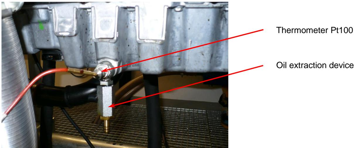
**Figure 4-4:** Oil sampling from the engine oil pan
