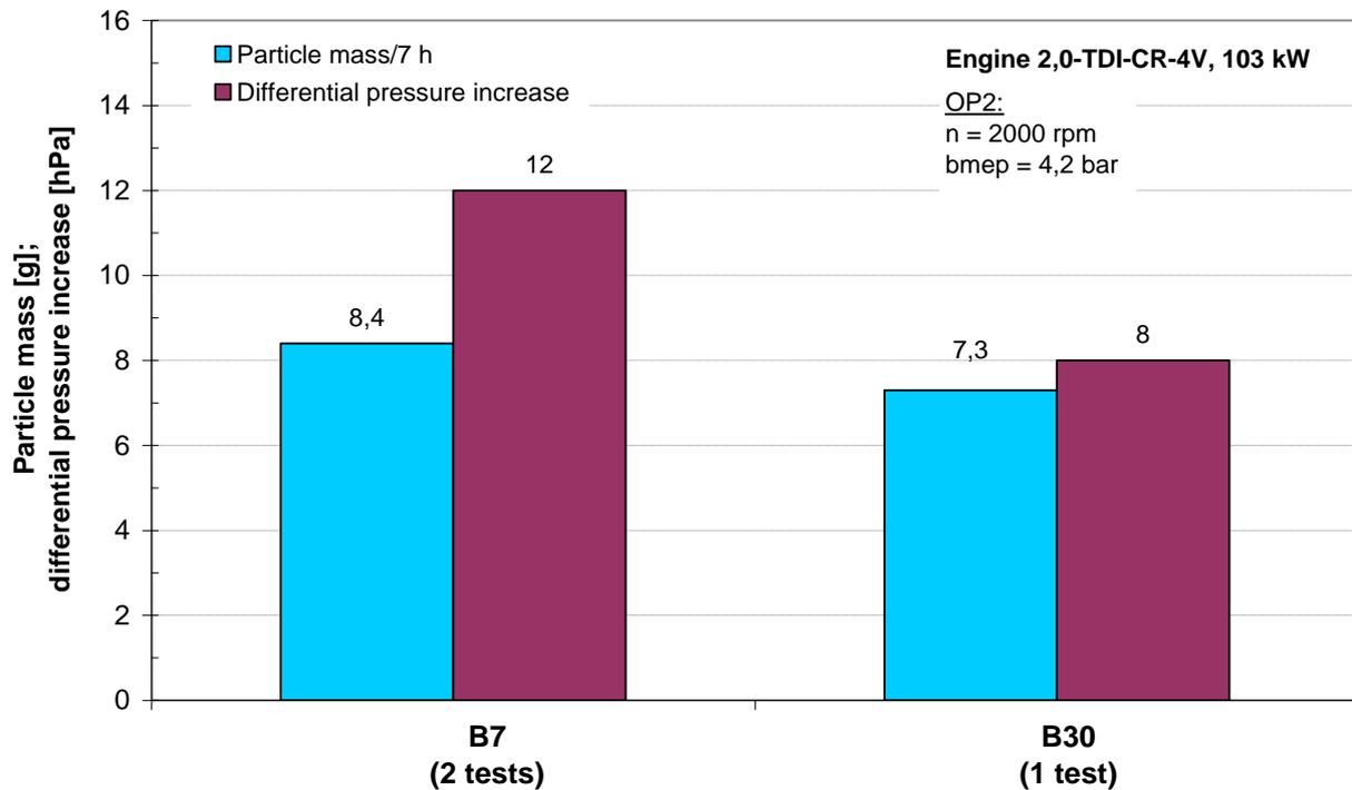
**Figure 6-15:** Accumulated particle mass and differential pressure of the DPF after charging the filter over 7 hours during engine operation at OP2 with B7 and B30
