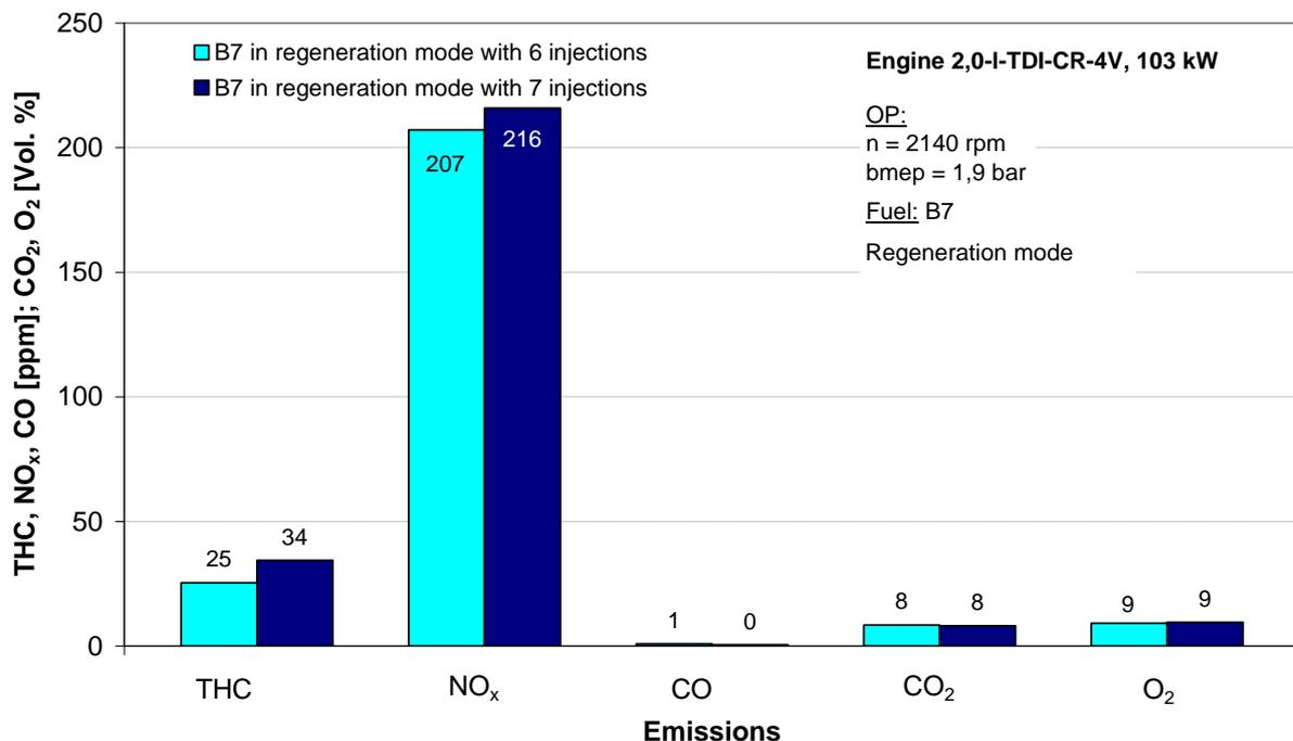
**Figure 6-18:** Exhaust gas emissions after DPF immediately before end of the regeneration of the particle filter during engine operation with B7 in regeneration mode with 6 and 7 injections per cycle at OP1
