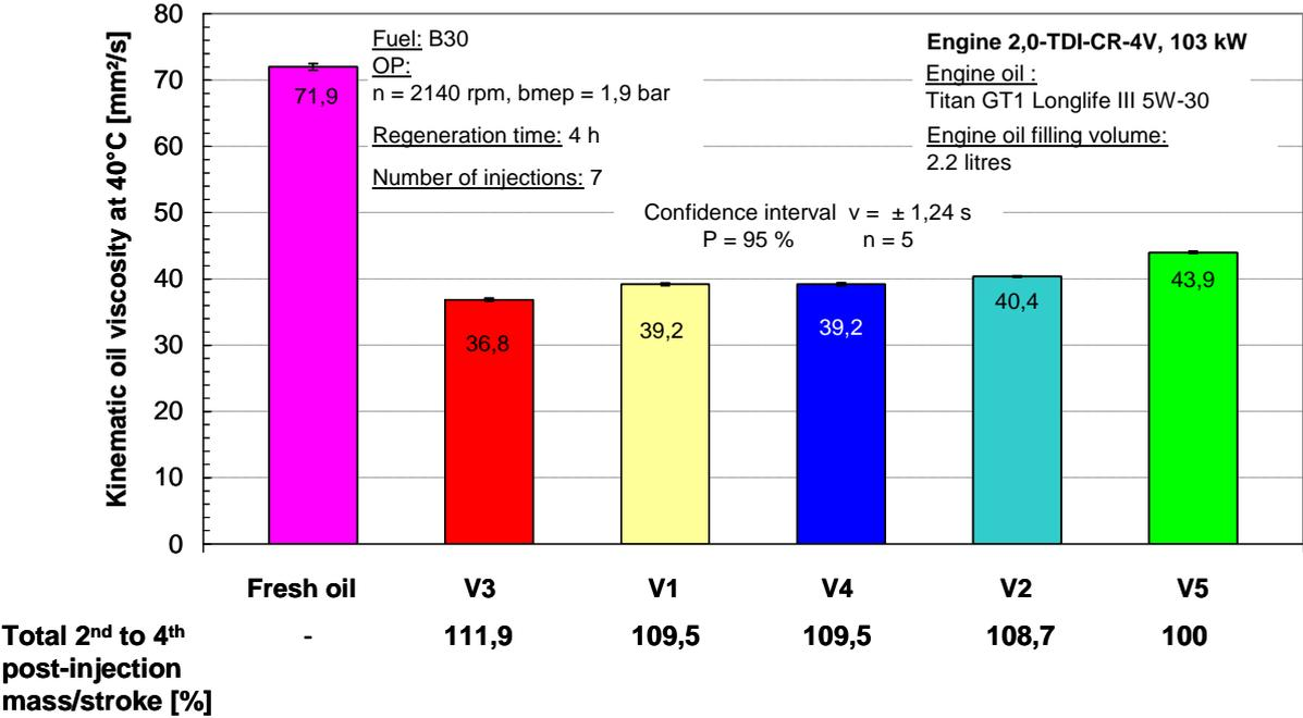
**Figure 6-3:** Kinematic oil viscosity at variation of the split late post-injection
