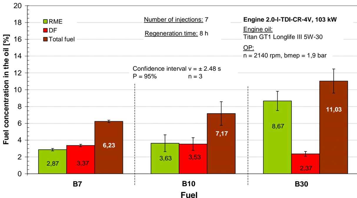
Figure 6-5: Concentration of total RME, DF and fuel in the engine oil after 8 hours engine operation in regeneration mode with 7 injections per cycle at OP1 with B7, B10 and B30
