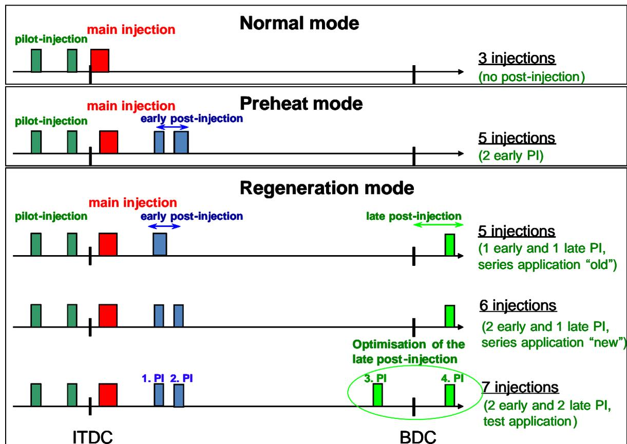
Figure 4-7: Injection sequence in normal, preheat and regeneration mode at OP1 for three different applications of the engine control unit
