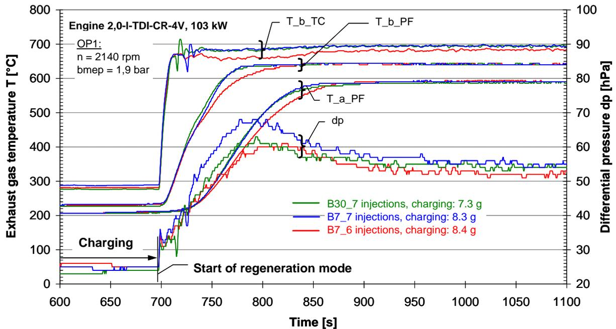
**Figure 6-16:** Regeneration of the particle filter during engine operation at OP1 with B7 and B30 in regeneration mode with 6 and 7 injections per cycle
