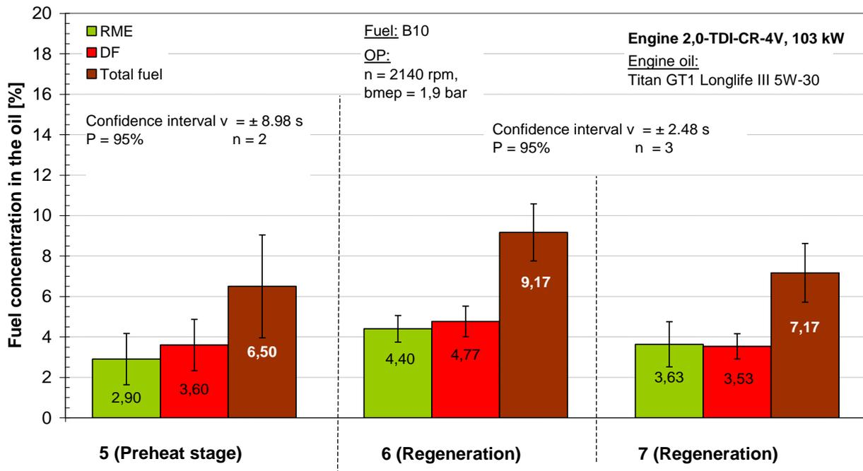
**Figure 6-11:** Fuel concentration in the engine oil after 8 hours engine operation with B10 in preheat mode with 5 injections and in regeneration mode with 6 and 7 injections per cycle at OP1
