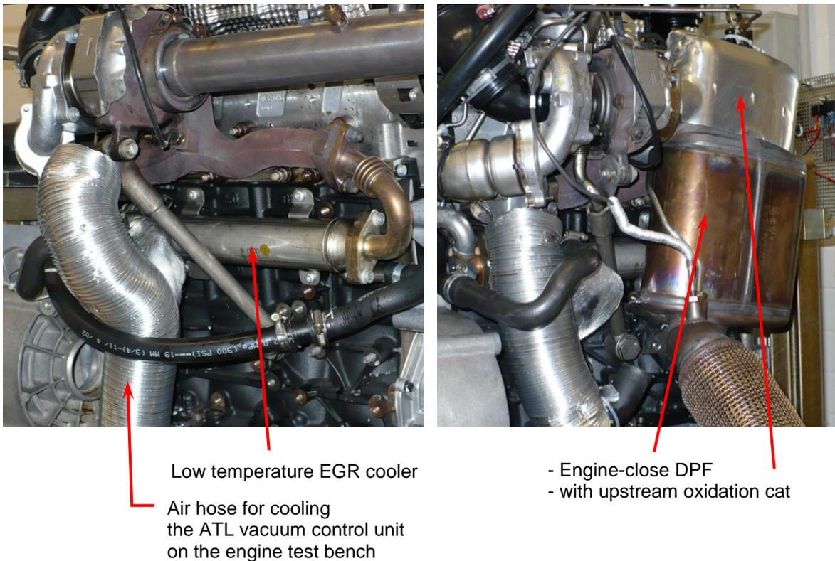
**Figure 4-1:** Low-temperature EGR cooler (left) and engine-close DPF with oxidation catalyst (right)
