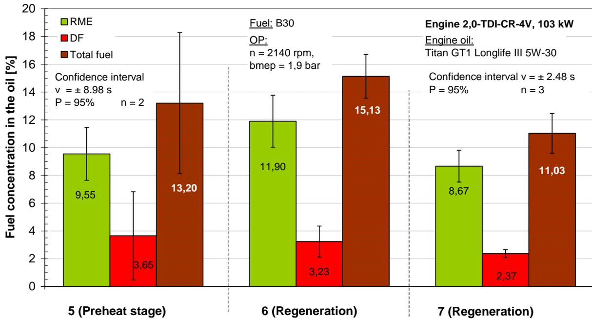
**Figure 6-12:** Fuel concentration in the engine oil after 8 hours engine operation with B30 in preheat mode with 5 injections and in regeneration mode with 6 and 7 injections per cycle at OP1
