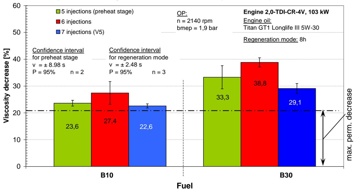
**Figure 6-13:** Decrease in the oil viscosity after 8 hours engine operation with B10 and B30 in preheat mode with 5 injections and in regeneration mode with 6 and 7 injections per cycle at OP1
