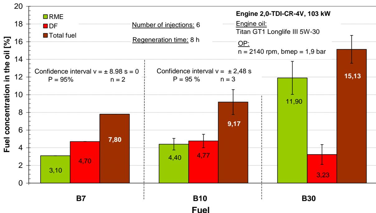
**Figure 6-4:** Concentration of RME, DF and total fuel in the engine oil after 8 hours engine operation in regeneration mode with 6 injections per cycle at OP1 with B7, B10 and B30
