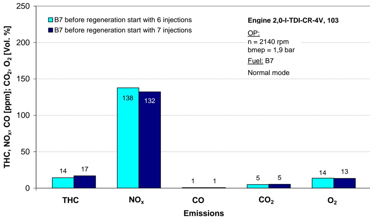
**Figure 6-17:** Exhaust gas emissions after DPF immediately before start of the regeneration of the particle filter during engine operation at OP1 with B7 in normal mode with 3 injections per cycle
