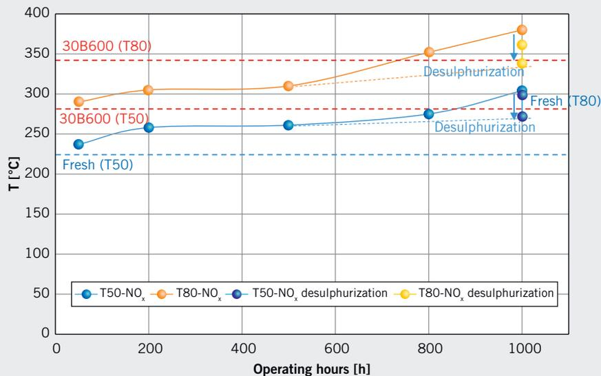
**FIGURE 7** T50 and T80 value of SCR performance throughout the operating time of 1000 h (© University of Rostock)
